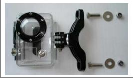
The GoPro camera mount hardware attachment to the front panel is as shown on the left. The same mechanical mounting method is able be adapted for use with most cameras.
